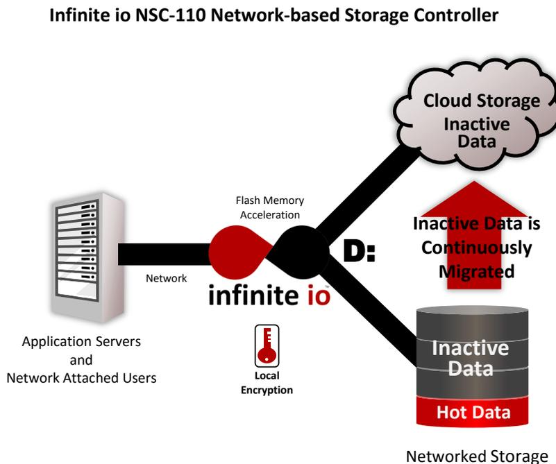
*The NSC-110 installs as a bump-on-a-wire and continuously migrates inactive data to an object store or cloud while being totally invisible to installed storage and applications*
